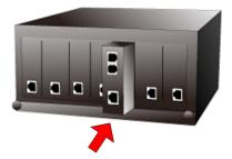
Figure 3-6: Insert a VDSL2 converter into an available slot
